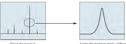
Detect the maximum level within full span.
