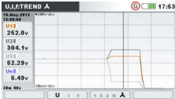
Image 0.16: Tendence de tension (toutes tensions)
