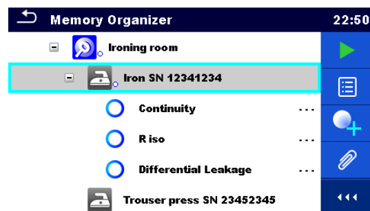
Figure 5.3: Example of status - No measurement result(s)
