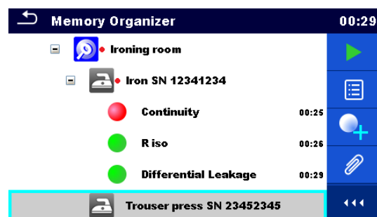
Figure 5.5: Status - Measurements completed with fail result(s)
