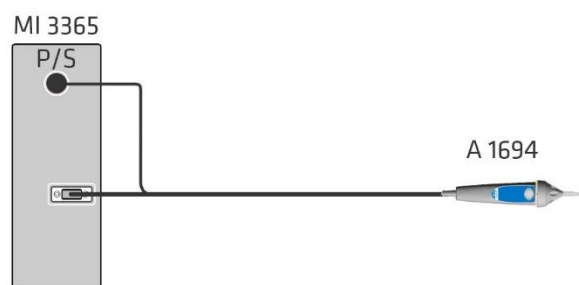
Figure 9.3: Raccordement du Tip Commander (A 1694)
