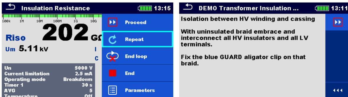
The offered options in the control panel depend on the selected single test, its result and the programmed test flow.
