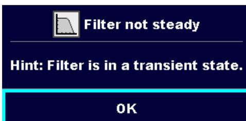
Filter (Average) is in transient state and needs additional samples.
