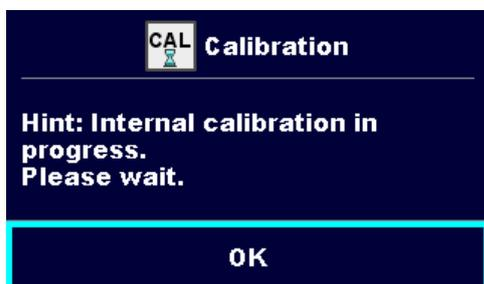
Instrument is in self-calibration mode. This is performed automatically after the instrument is powered-on and lasts a few seconds.
