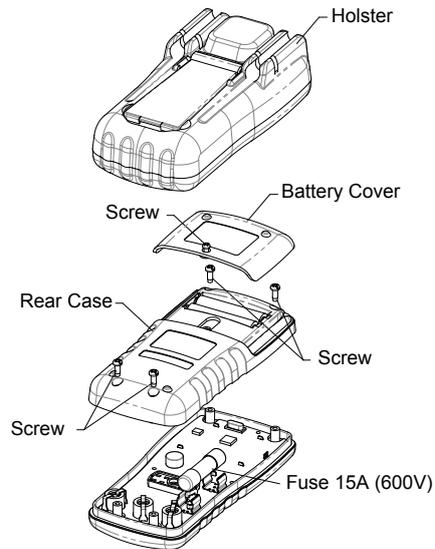
**Fuse type : 15A/600V – 50KA (10x38mm)**
