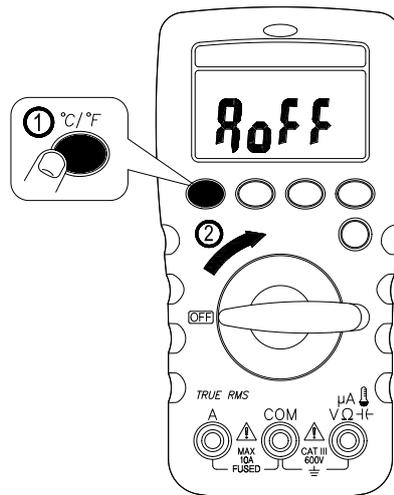
Dial the switch to off position ,then keep the Function button down and turn the meter on.
