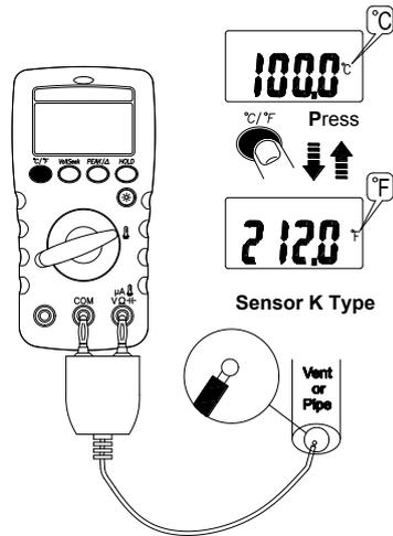
Dial the switch and press the Function button to select the measuring function. (°C / °F)
