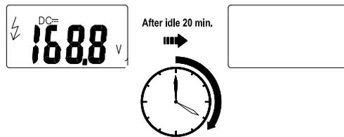
Wake-up the meter by dialing the switch or pressing any button.
