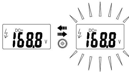
Press the Backlight button to turn the backlight on/off.
