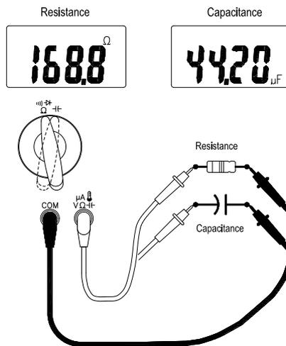
Dial the switch and press the Function button to select the measuring function.
