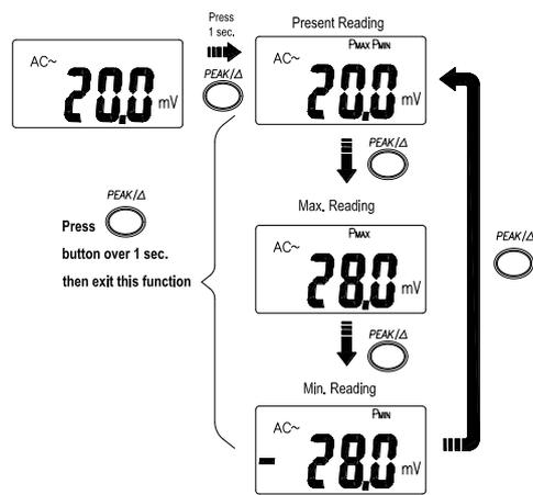
In the Peak Hold function ,the meter records the peak min. value and the peak max. value when the inputs goes below the recorded peak min. value or above the recorded peak max. value, the meter records the new value . Press Hold button to pause the recording.
