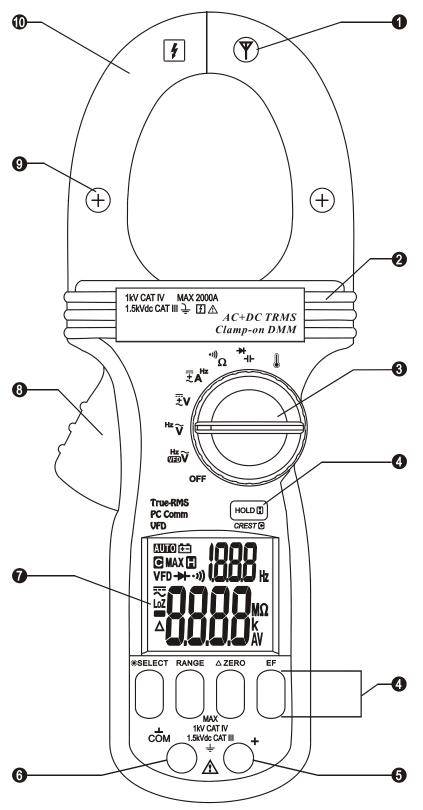
1) Antenna for Non-Contact EF-Detection
