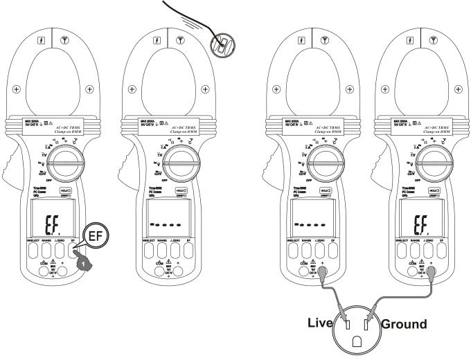
•Non-Contact EF-Detection: An antenna is located along the top-right end of the clamp jaw, which detects the electric field surrounds energized conductors. It is ideal for tracing live wiring connections, locating wiring breakage, and distinguishing between live or earth connections.
