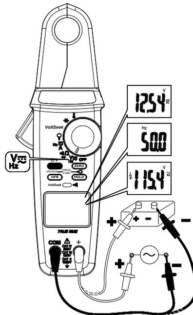
Dial the switch and press the Function button to select the measuring function.
