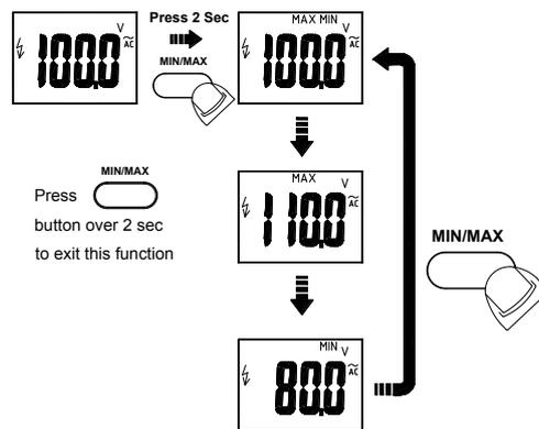
In the MIN MAX function ,the meter records the min value and the max value .
