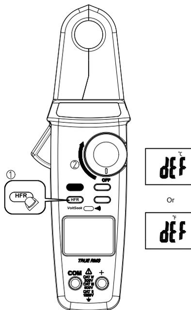
Dial the switch to off position, then keep the HFR button down and turn the meter on.
