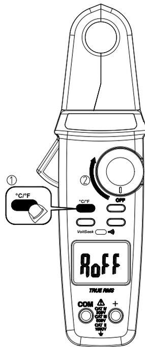
Dial the switch to off position, then keep the Function button down and turn the meter on.
