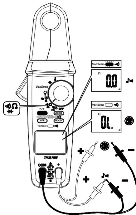
Dial the switch and press the Function button to select the measuring function.
