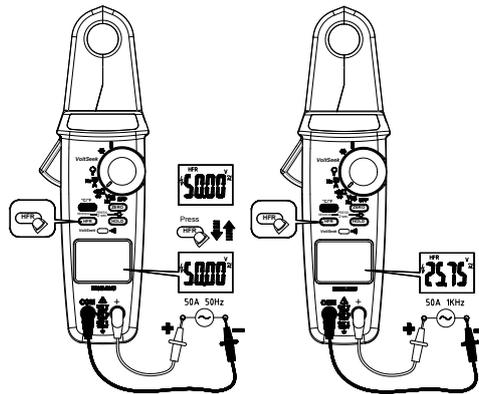
The Cut-Off frequency of the low pass filter is about 800Hz with attenuation characteristic of approx. -24dB/octave.
