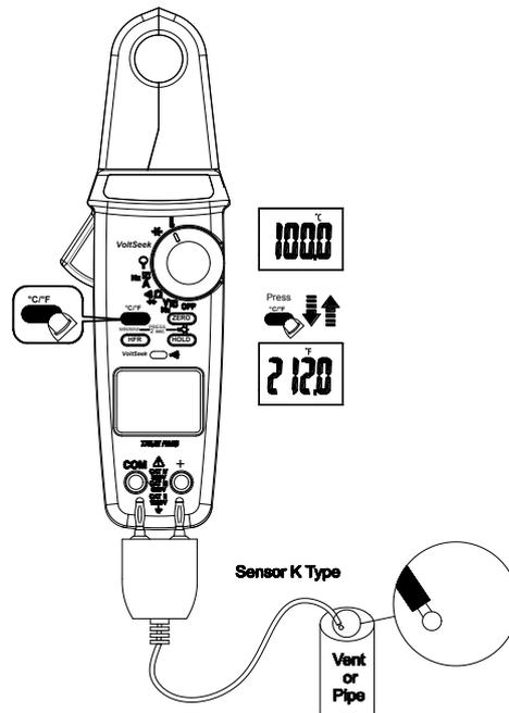
Dial the switch and press the Function button to select the measuring function. (°C / °F)
