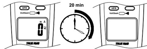
Wake-up the meter by dialing the switch or pressing any button.
