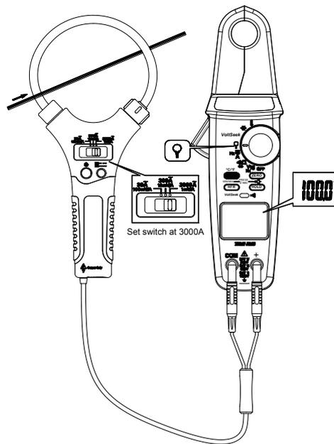
Dial the switch to select the measuring function.
