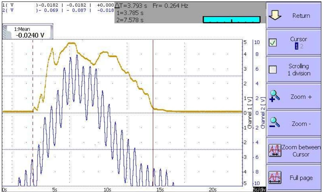
It is possible to trigger on a periodic signal parasite (50 Hz-main): the trigger is executed when the signal shape changes radically.
