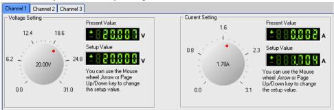
Use the mouse to click on the rotary knob and move the mouse to change the value. You also can use the mouse wheel, or Page Up/Down keys and arrow keys  $(\uparrow, \downarrow, \leftarrow, \rightarrow)$  from the keyboard for fine adjustment of voltage or current values. The setup value will be displayed on the second line indicator.
