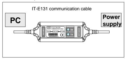
**Note:** It is **not possible** to connect the DB9 connector of the power supply directly to a PC's RS232 or USB port.
