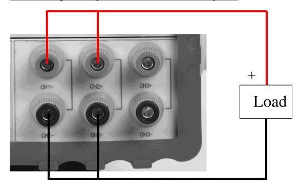
Note: When configuring for series or parallel operation, the user must wire the terminals to match the configuration. The power supply does not automatically connect the appropriate terminals internally based on the configuration selected.
