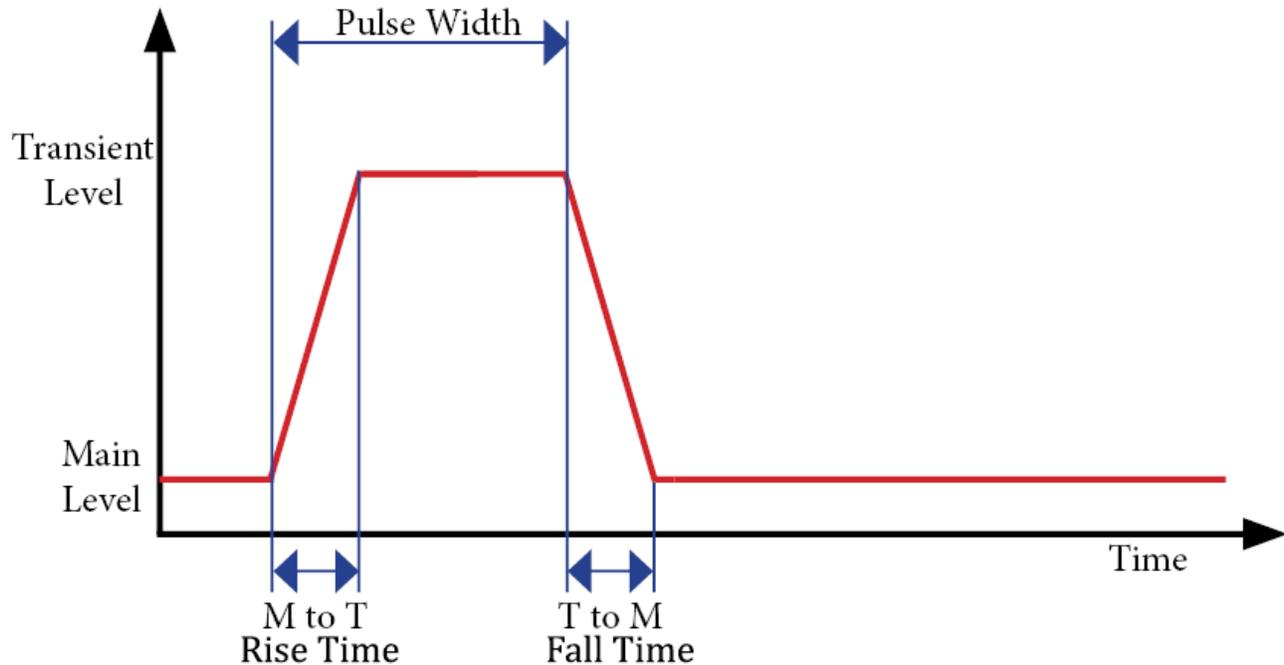
Figure 6.6 Pulse Transient Mode
