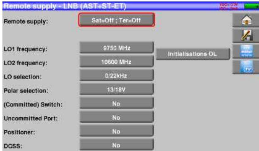
The window allows you to select the remote power supply on terrestrial and/or satellite mode.
