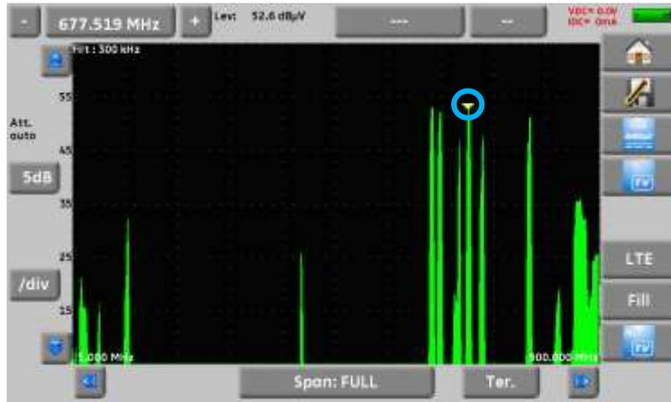
Press the NIT/TV key
