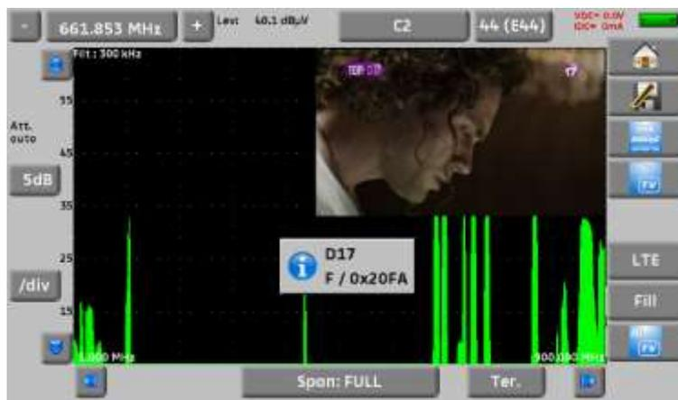
Press the Measures-TV-Spectrum key. You can now display the level, the BER/MER, the TV detection (with information about the current service) and the spectrum of the signal selected on the same page...
