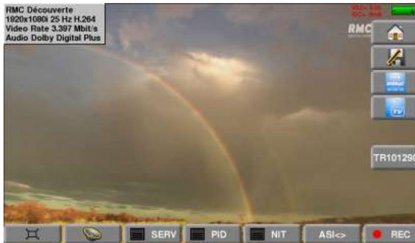
The instrument analyze in real time, the Transport Stream (TS) from the RF input or the ASI input, according the DVB recommendation TR101290 defining an Alarms list.
