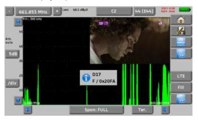
Press the Measures-TV-Spectrum key. You can now display the level, the BER/MER, the TV detection (with information about the current service) and the spectrum of the signal selected on the same page...
