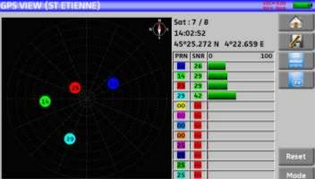
When satellites have been found, they appear on the pattern; non-locked satellites blink.
