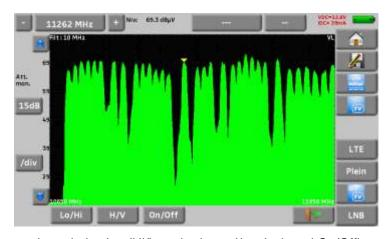
LNB function: to change the polarization (Hi/Low, horizontal/vertical, and On/Off)
