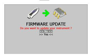
Move the highlighted line (reverse video) with up/down keys of the sensitive wheel, and then press the central key: the updating process is running
