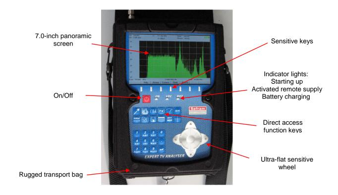
The front panel is equipped with an ultra-flat sensitive wheel with direction keys. For selection keys see below.
