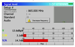
The appliance tries to perform a level measurement out of these possibilities (for example an Audio measurement with an 865 MHz video carrier).
