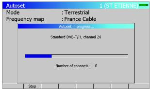
7/ once the search is completed, the appliance automatically goes to the Measurement Map mode. It displays different measurements (Level, MER...) for the found setups.
