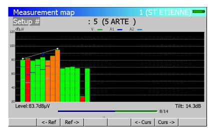
The **audio carriers**' levels are added on the associated video carrier histogram, according to the colours in the legend at the top and on the right of the page.
