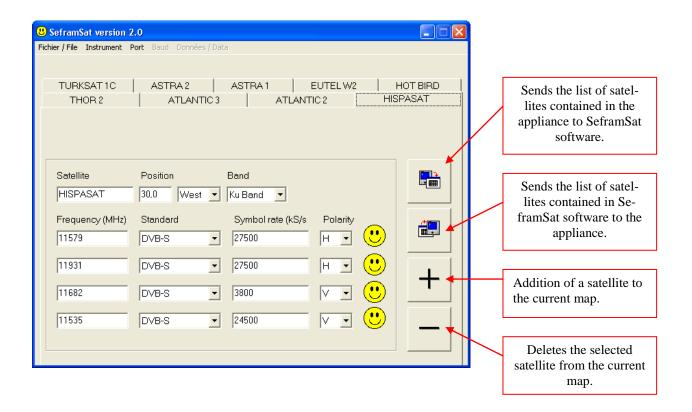
**SeframSat** permits to characterise completely one or several satellites: each parameter can be modified either directly by keyboarding its value or by selecting from a drop-down list.
