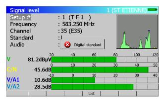
2<sup>nd</sup> press on the level key: The appliance tries to perform an error rate measurement with a **Standard** different **DVB-C**, **DVB-S**, **DVB-S2**, **DSS or DVB-T/H**.
