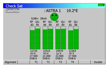
The appliance has 30 pre-programmed satellite orbital positions in storage. Each satellite possesses 4 transponders.
