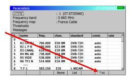
Select the file to be copied using up and down keys and then, press the « Copy » button.
