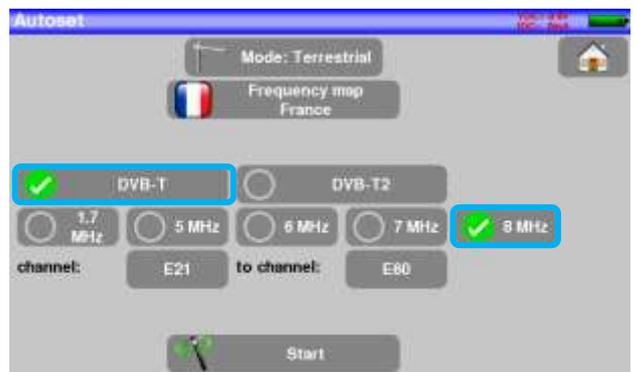
Press START. The appliance searches until the end of the scan and turns directly to the Measures page. If no channel has been found, see the next chapter.
