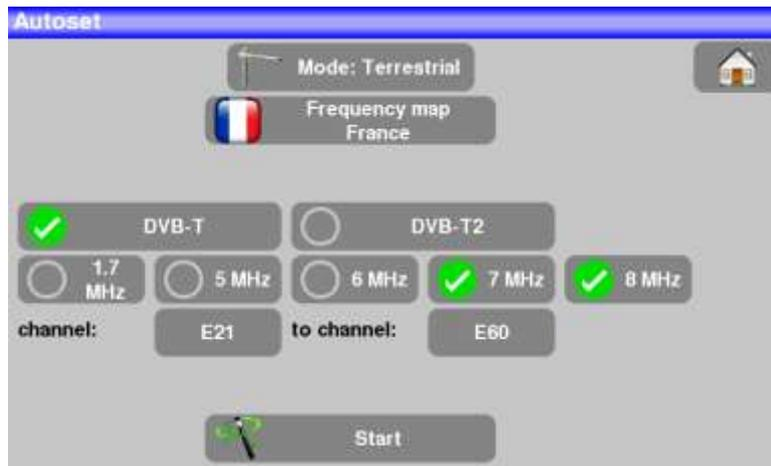
A green check shows that the parameter is included in the research. If there is no green check, the parameter will not be taken into account for the research.
