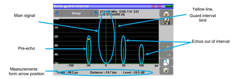
Relative amplitude in dB and delay in µs (distance in km) from the main signal (0 pulse) can be measured.
