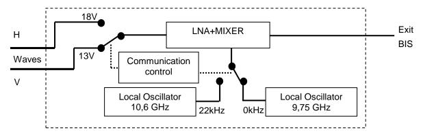
The reception is made on 2 low/high frequency band and 2 horizontal/vertical polarizations of the received wave.
