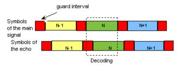
You have to reduce the level of reception of the echoes by orienting the antenna or by selecting a more directive antenna.
