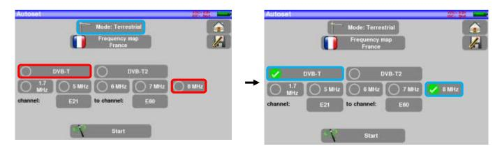
Press START. The appliance searches until the end of the scan and turns directly to the Measurement plan mode. If channels were found, the appliance makes measurements continuously (C/N-level, then BER/MER) on the detected channels. If no channel has been found, see the next chapter.
