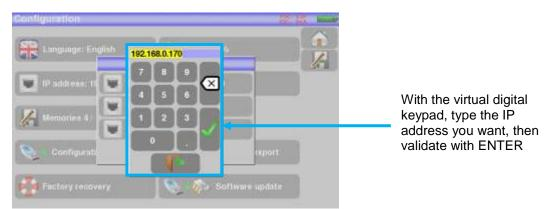
The PC software in communication with the appliance must have the same IP address as the appliance, just like in the example below:
