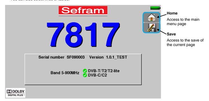
The Home page allows the navigation through all functions of the appliance. You will also find there the <u>Remote supply</u> and <u>Measures-TV-Spectrum</u> functions, the <u>AUTOSET</u>, <u>Lists</u>, <u>Library</u>, <u>TERRESTRIAL check</u>, <u>Configuration</u>, <u>Constellation</u>, <u>Echo Guard Interval</u> and <u>Measurement map</u>.
