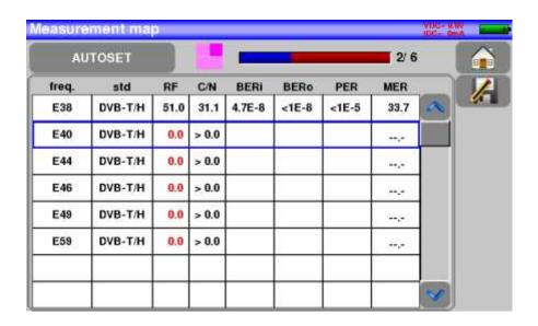
Any detected channel will be registered into the first empty list (automatically renamed AUTOSET) **and** into the fist available setups of the library, starting from the end of the table.
