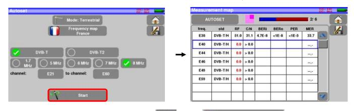
To finish, press the home measurement key press Prog, select the channel that you want to display.
