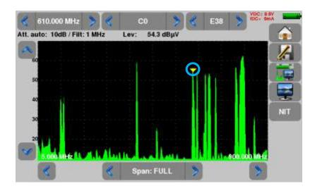
Press the NIT key, the device find automatically all the parameters of the signal.
