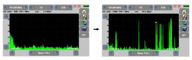
Press directly the signal you want in the spectrum (the cursor moves to where you press)
