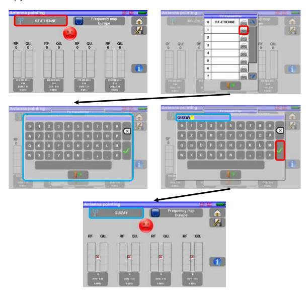
Enter 4 frequencies or channels of the transmitter you try to check.
