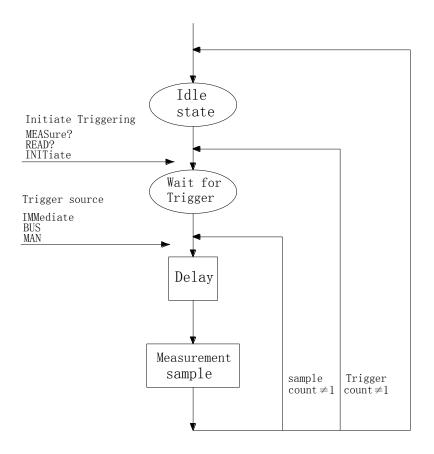
Figure 4-2 Trigger model
