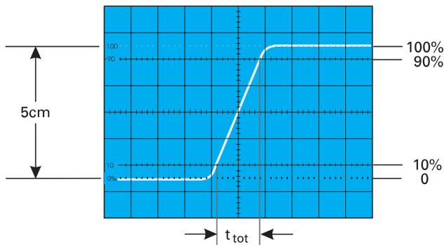
With a time coefficient of  $5\text{ns}/\text{div}$  (X x10 magnification active), the example shown in the above figure results in a total measured rise time of
