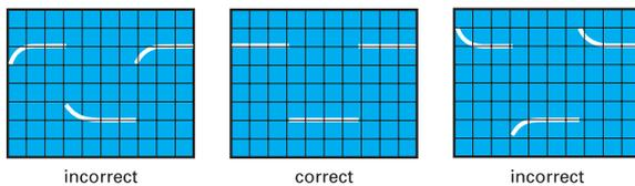
Connect the probes to the CH I input. Set the deflection coefficient to 5mV/div and the input coupling to DC. The time deflection coefficient should be set to 0.2ms/div. All deflection coefficients should be calibrated. Plug the probe tip into the calibrator output socket.
