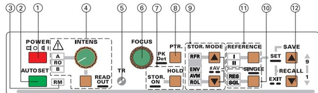
(9) **RFR** - stands for refresh operation. In this mode, as in analog mode, periodically repeating signals can be captured and displayed.
