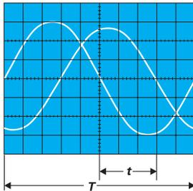
and possibly also using the time vernier (variable) adjustment.
