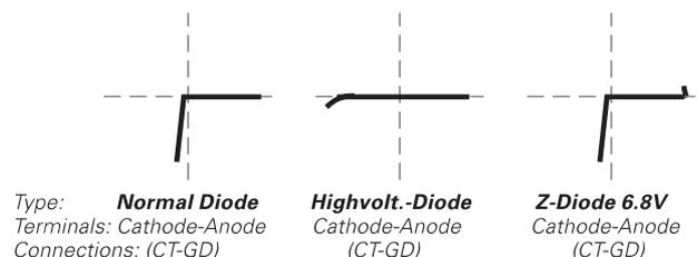
The polarity of an unknown diode can be identified by comparison with a known diode.
