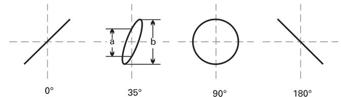
Calculation of the phase angle or the phase shift between the X and Y input voltages (after measuring the distances a and b on the screen) is quite simple with the following formula, and a pocket calculator with trigonometric functions. Apart from the reading accuracy, the signal height has no influence on the result.
