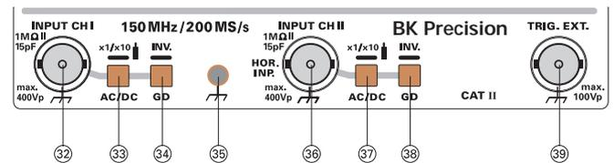
**(33) AC / DC** - Pushbutton with two functions.
