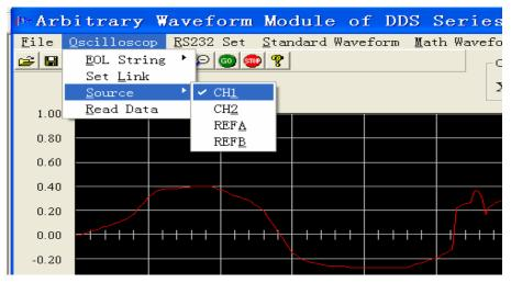
7) Read the oscilloscope data from the source selected: Click on "read data" in sub-menu oscilloscope". A pop-up window will appear to display the current status of the transfer. The pop up window will automatically disappear once transmission was completed successfully and the downloaded data will automatically be displayed in the Software's editing window.
