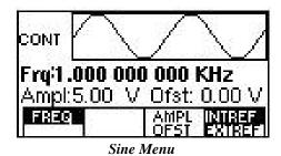
F1: FREQ - (Frequency) Selects and displays the frequency. Change the frequency setting using the cursor keys and rotary knob or numerical keypad. If a certain wavelength can't produce the waveform at the desired frequency, the waveform generator displays an "Out of Range" error message.
