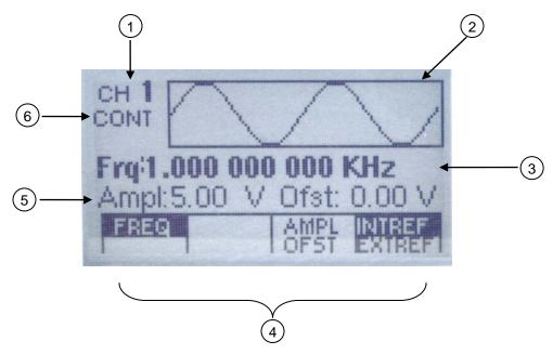
Figure 3.2 - LCD Display Screen
