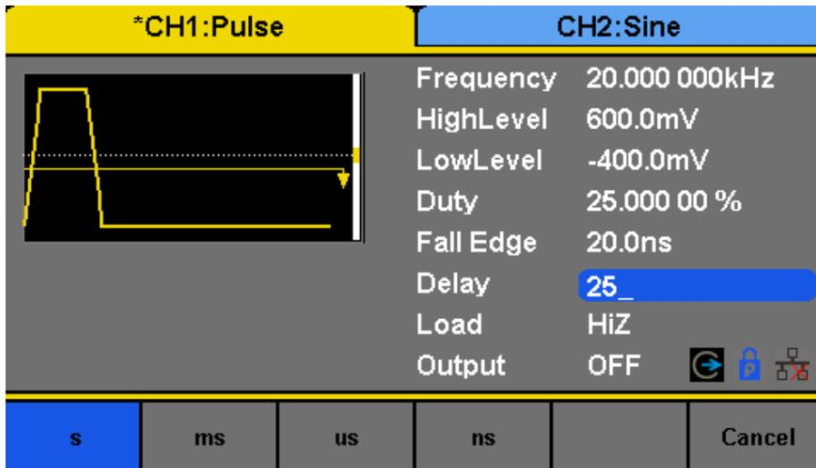
Figure 5.10 Pulse Delay
