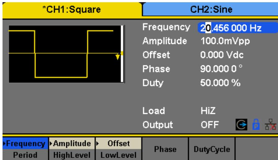
**Figure 3.1** Square Wave Parameters
