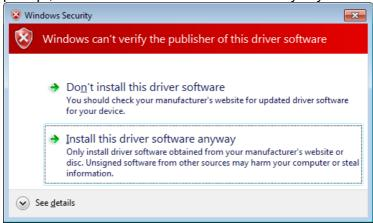
12. The driver will now install. Once finished, under "Device Manager", you should see under "Ports (COM & LPT)" an item labeled "BK Precision USB to Serial Converter (COM#)". The "COM#" is the com port that can be used to access the virtual COM port for remote communication.
