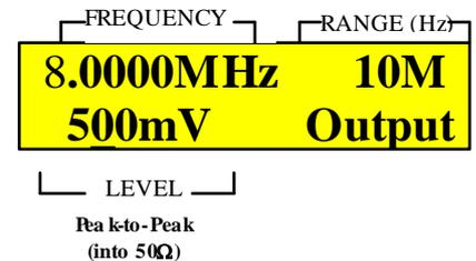
Figure 15: LCD example of using -20dB attenuation
