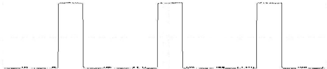
Example of symmetric square wave, duty cycle set to 50%.
