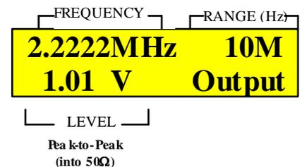
Figure 11: LCD example of using fifth frequency range
