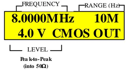
Figure 17: LCD example of displaying CMOS output level
