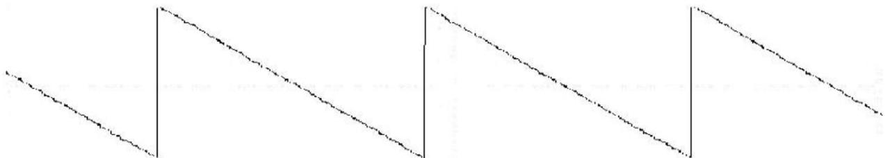
Example of ramp wave (asymmetric triangle), duty cycle set to 20%.
