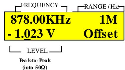
Figure 7: LCD example of displaying offset parameter
