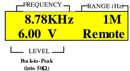
Figure 28: LCD example of displaying frequency when in REMOTE mode
