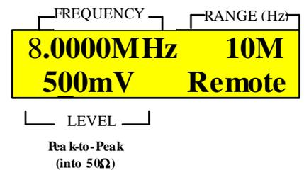
Figure 29: LCD example of sweep start frequency in REMOTE mode
