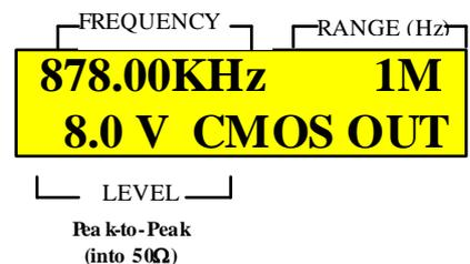
Figure 8: LCD example of displaying CMOS output level
