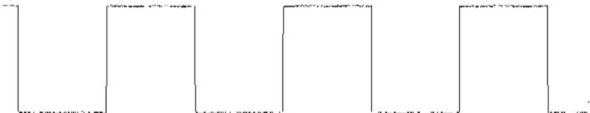
Example of asymmetric square wave (pulse), duty cycle set to 70%.
