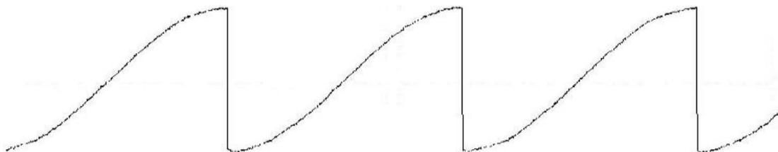
Example of asymmetric sine wave, duty cycle set to 20%.
