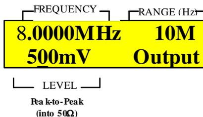
Figure 20: LCD example of sweep start frequency
