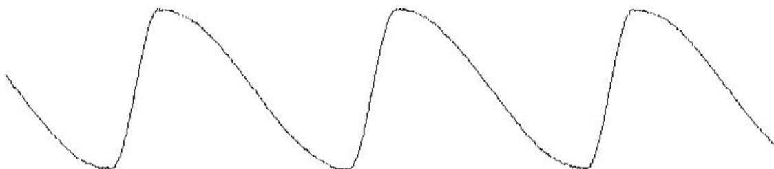
Example of asymmetric sine wave, duty cycle set to 100%.
