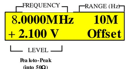
Figure 16: LCD example of displaying offset parameter
