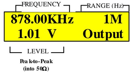
Figure 4: LCD example of using fourth frequency range
