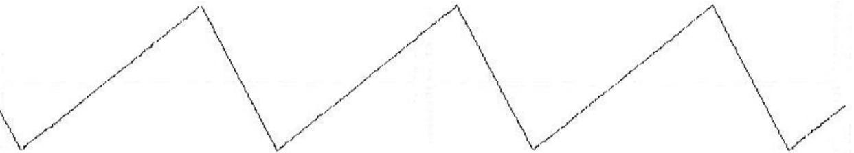
Example of ramp wave (asymmetric triangle), duty cycle set to 100%.
