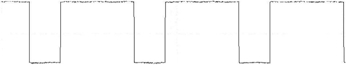
Example of asymmetric square wave (pulse), duty cycle set to 95%.
