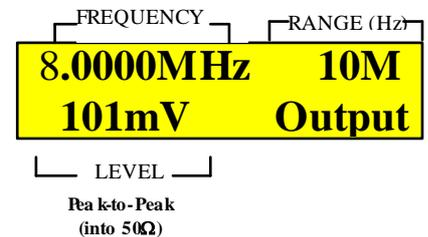
Figure 14: LCD example of using -20dB attenuation
