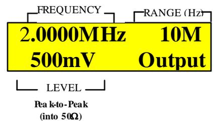
Figure 21: LCD example of sweep stop frequency
