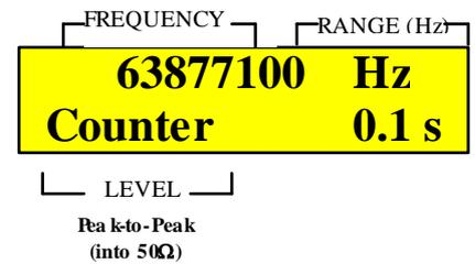
Figure 23: LCD example of displaying measured frequency using 0.1 s gate period time
