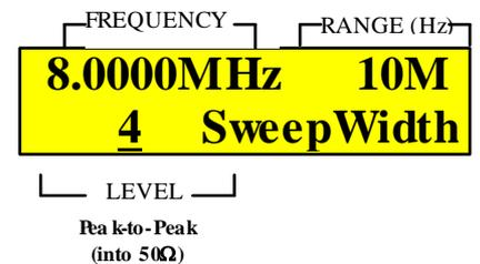
Figure 18: LCD example of displaying sweep width parameter
