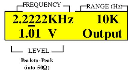
Figure 2: LCD example of using second frequency range
