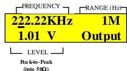
Figure 3: LCD example of using fourth frequency range
