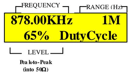
Figure 5: LCD example of displaying duty cycle parameter
