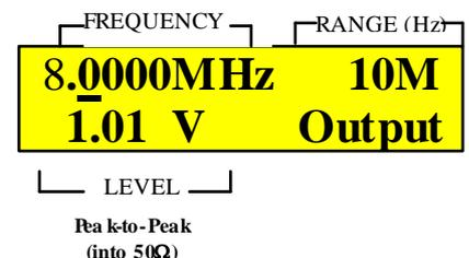
Figure 12: LCD example of using fifth frequency range
