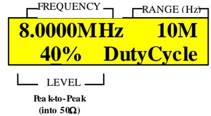
Figure 13: LCD example of displaying duty cycle parameter
