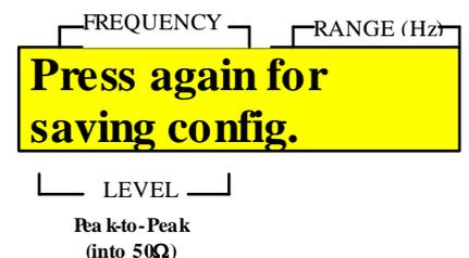
Figure 25: LCD example of displaying the initialization of saving current configuration
