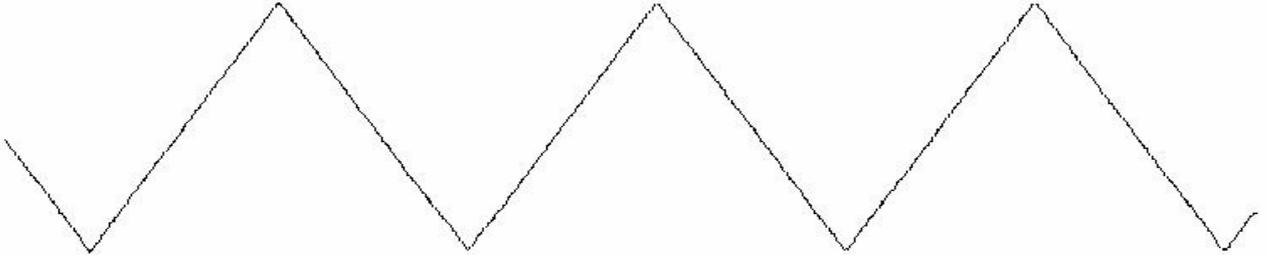
Example of ramp wave (asymmetric triangle), duty cycle set to 70%.
