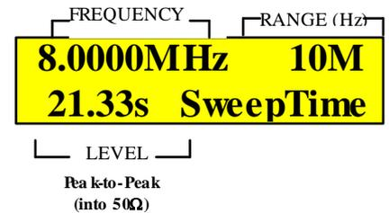
Figure 19: LCD example of displaying sweep time parameter
