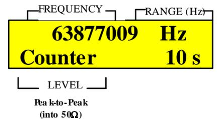
Figure 24: LCD example of displaying measured frequency using 10 s gate period time
