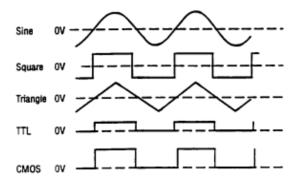
Figure 2. Output Waveform and Phase Relationship
