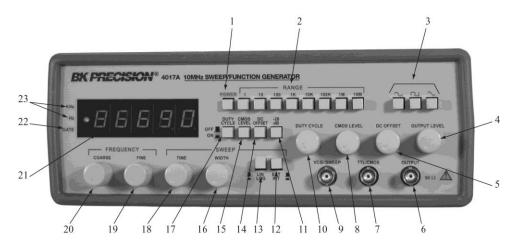
Figure 1. Model 4017A Front Panel.
