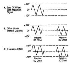
Figure 3. Use of DC OFFSET Control
