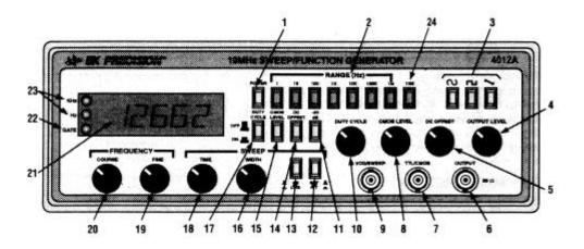
Figure 1. Model 4012A Front Panel.
