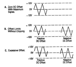
Figure 3. Use of DC OFFSET Control
