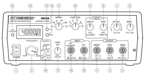
Figure 2 - Front Panel Controls (4003A)
