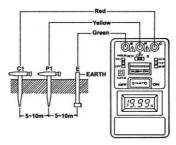
3. Set the Range Switch to suitable range and set the function switch to position then press the PUSH-ON BUTTON and TIMER ON BUTTON at the same time and take the reading on the display.
