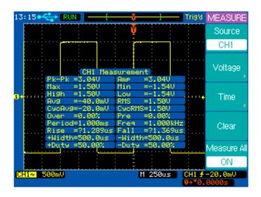
Press the **Measure All** softkey again to turn off Auto Measurements.
