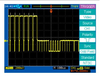
Trigger on a Specific Line or All Lines of the Video Signal
