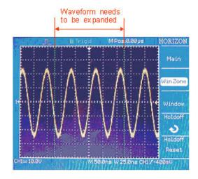
Figure 3-19 Window setup
