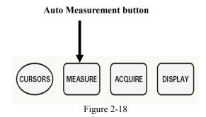
Press the 'MEASURE' button. There are 11 types of measurements available. You can display up to five measurements at a time. To define each of the 5 measurements, do the following:
