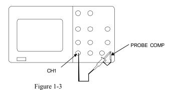
3. Press the "AUTO" button. After a few seconds, you should see a square wave signal with a 1KHz frequency and about 3V peak-peak amplitude
