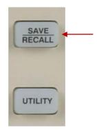
The scope can save 2 groups' reference waveforms, 20 groups' setups, and 10 waveforms to the oscilloscope's internal memory. There is a USB Host interface in the front panel of the oscilloscope where you can save setup data, waveform data, waveform interface image, CSV file to a USB flash drive. Setup data and waveform data can be recalled to the oscilloscope. Picture data and CSV file can't be recalled to the oscilloscope, but it can be opened on a computer.
