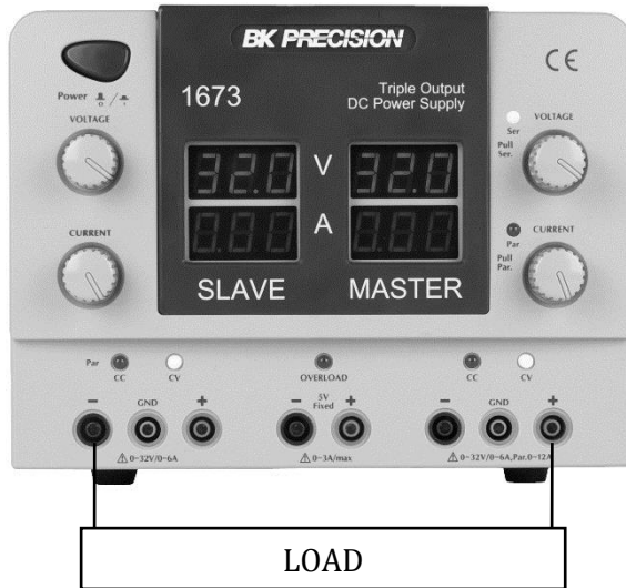
Figure 5 – Series Tracking Mode Load Connection
