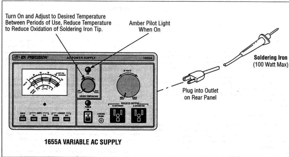
Figure 13. Using the Variable Soldering Iron Temperature Feature.
