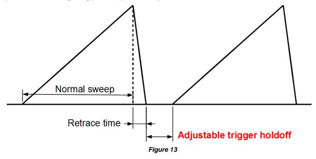
This holdoff adjustment can be valuable in helping you trigger on signals that would otherwise be difficult to trigger on.
