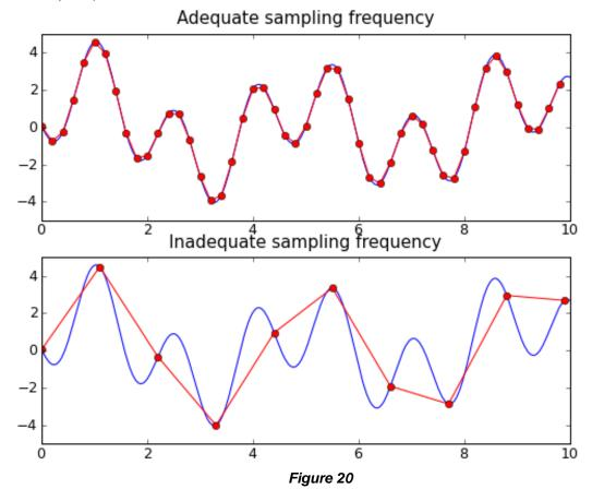
The "Adequate sampling" samples reproduce the waveform adequately. With some suitable low pass filtering, this could be an excellent reconstruction of the original waveform. However, the "Inadequate sampling" reconstruction **misses important details in the waveform**. With some low pass filtering to remove the sharp corners, you'd probably conclude the original waveform was about one-third the frequency of the actual waveform. Other waveform measurements would be in error too.
