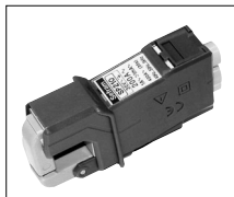
SP201 : 200 AAC, 10mV/1A, ø 15 mm.
