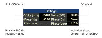
Set voltage, frequency, and phase directly from the front panel on each AC source.
