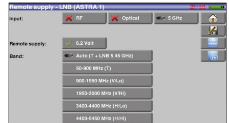
5.4GHz input: band selection and remote supply control
