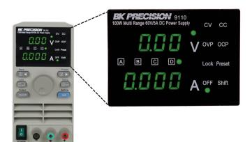
The 9110 is a new type of power supply. Unlike conventional power supplies with fixed output ratings, the 9110 automatically recalculates voltage/current limits for each setting. The 9110 provides 100 W output power in any Volt/Amp combination within the rated voltage (60 V) and current (5 A) limits. By providing greatly expanded choices of maximum power Volt/Amp combinations, users can cut down on the number of power supplies required and free up valuable bench space.
