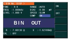
Quickly sort components using the instrument's 9 primary BINs, a secondary BIN and out-of-specification BIN. The results can be displayed in a table on-screen or output via the handler interface. High and low limits for each bin can be set up in absolute, tolerance or sequential mode with Pass/Fail indicator.
