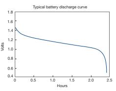
Built-in battery test function to calculate the Ah characteristic and capacity of a battery using a fixed current load discharge. Specify stop conditions for cut-off voltage, capacity level, and time up to 27 hours. Programmable DC Electronic Loads 8500B Series
