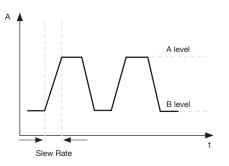
Transient operation to periodically switch between two load levels. A power supply's regulation and transient characteristic can be evaluated by monitoring the supply's output voltage under varying combinations of load levels, frequency, duty cycle, and slew rate. These combinations are all controllable in the continuous, pulse, and toggled modes.
