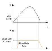
Control the input turn on state for the DC electronic load by configuring the Von latch functions. This can be used to start and stop discharging of a battery or other power source once a specified voltage level is reached.
