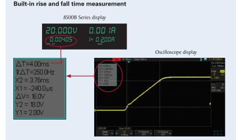
The 8500B Series can measure the rise or fall time from a specified start and stop voltage level of the measured input without the need for an oscilloscope. This function can also be used as an internal timer to count how long the input has been enabled.
