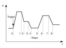
List mode lets you generate more complex sequences of input changes with several different levels. Save up to 7 groups of list files to internal memory for recall and set parameters including step counts (range 2 to 84), width time of a single step (minimum 20  $\mu$ s), step value, and slope.
