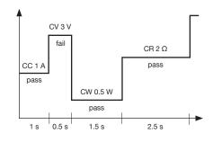
Execute multiple test sequences in automatic test mode. Up to 100 different sequences can be linked to run steps of various operating modes and load conditions.
